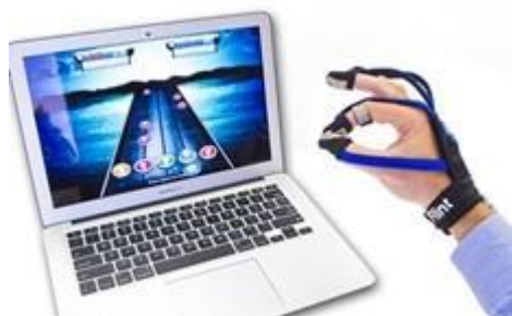
Fig. 1. MusicGlove: An interactive device paired with a PC or tablet, featuring conductive fingertip pads to detect finger movements. It prompts users to perform timed grips in sync with scrolling notes descending on a computer screen.
